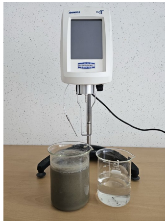
Fig. 1 Experimental setup for viscosity evaluation
